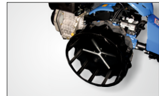
metal grid wheels, special CaneThumper attachment for operating on steep slopes
