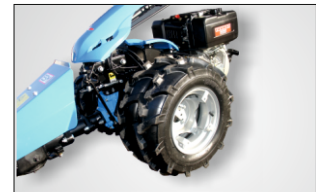
twin tyres, special CaneThumper attachment for operating on slopes
